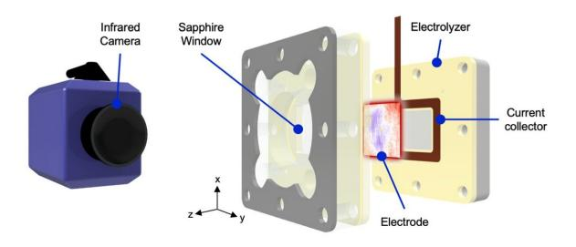
By using an infrared camera, the research team can detect the distribution of electrons on the electrode. Using these insights, they then designed a new way of delivering these electrons more evenly over the surface. Credit: Delft University of Technology
