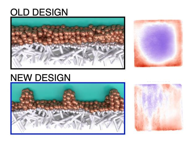
The researchers designed a new way of delivering electrons more evenly over the surface of the electrode. In the left part of the illustration, the brown spheres are the copper catalyst, the white rods below represent the electrode and the blue arrows show the flow of current. On the right side, the purple spots are the cooler areas and the orange coloured hot spots show where the most current is. Credit: Delft University of Technology
