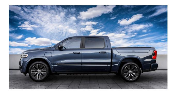
A 2025 Ram 1500 Ramcharger Tungsten is shown in this undated photo provided by Stellantis. Stellantis' Ram brand may have an answer for people who fear running out of juice on the road with nowhere to recharge. The Ramcharger, a pickup that can travel 145 miles on electricity with a V6 gas-powered generator that can recharge the battery while the truck is moving. Credit: Stellantis via AP
