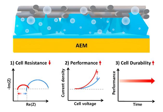
Figure 1. The first facile in-situ, ionomer-free catalyst-coated membrane (modified CCM; m-CCM) fabrication method, developed by the research team. Credit: *ACS Energy Letters* (2023). DOI: 10.1021/acsenergylett.3c01418
