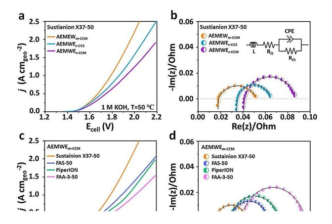
Figure 2. Electrochemical analysis of AEMWEs in 1 M KOH at 50 °C., as well as the long-term stability test of AEMWEs fabricated using an m-CCM, a c-CCS, and a c-CCM with Sustainion X37-50 at sequentially increasing constant current densities of 100, 500, and 1000 mA cm<sup>-2</sup>. Credit: *ACS Energy Letters* (2023). DOI: 10.1021/acsenergylett.3c01418
