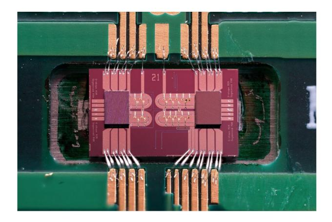
Photograph of PAM-4 transmitter comprising two CMOS electronic drivers flipchip bonded onto a silicon photonic modulator. Credit: Li et al.
