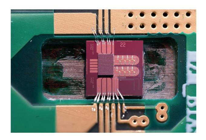
Photograph of OOK transmitter comprising a CMOS electronic driver flip-chip bonded onto a silicon photonic modulator. Credit: Li et al.
