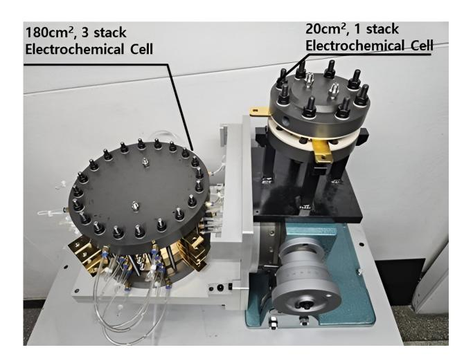
Photograph of trial product of the environment-friendly electrochemical refrigerant compressor. Credit: Korea Institute of Machinery and Materials (KIMM)
