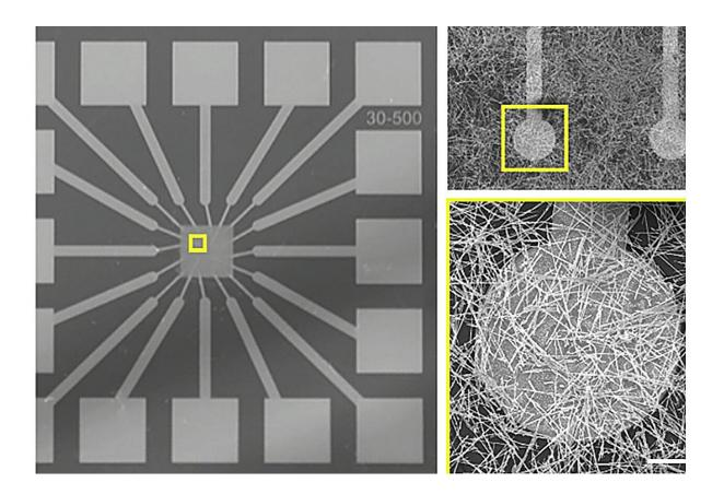
The new platform technology modeled after the brain is composed of a tangledup network of wires containing silver, laid on a bed of electrodes. Credit: Sam Lilak/UCLA
