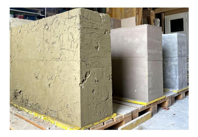
Prototype walls made with a clay, lime and cement. Credit: EPFL / Salvatore Aprea
