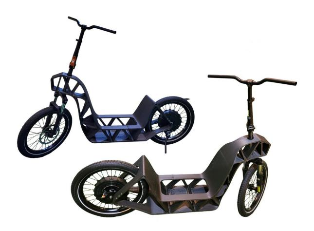
DynaLight Project: Load-bearing frame construction for the electric cargo scooter from the 3D printer. Credit: Fraunhofer IWU
