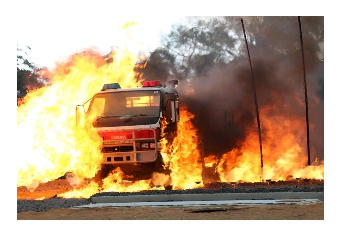
CSIRO testing of firefighting vehicles to support development of crew protection systems. Credit: CSIRO
