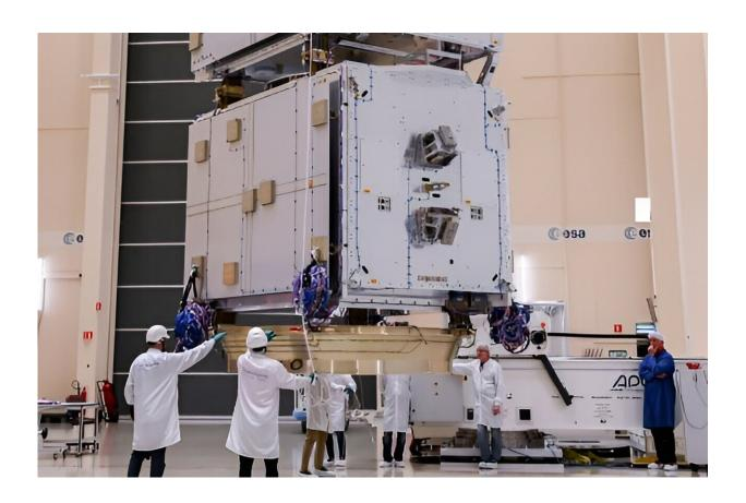
Galileo Second Generation satellites will be launched in pairs, interconnected and connected to the launcher until separation. Each satellite weighs more than 2,000 kg and when stacked they reach a towering height of seven meters. Credit: ESA-SJM Photography
