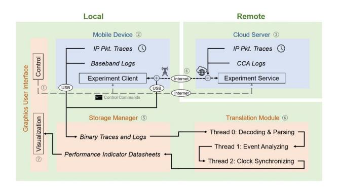
The black line with the arrow shows how traces and logs of carried network experiments are created, transferred, processed, and finally visualized as network performance indicators. Credit: Ruihan Li, et al
