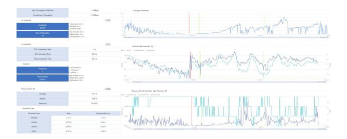
The top graph shows throughput metrics in the transport layer. The middle and bottom graphs prominently display variations in signal strength and resource allocation in the physical and data link layers. Handovers are included in all three graphs, providing a holistic view of network dynamics. Credit: Ruihan Li, et al
