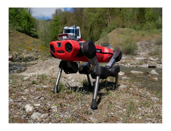
ANYmal is a four-legged robot for the inspection and maintenance of technical systems. Credit: Robotic Systems Lab / ETH Zurich
