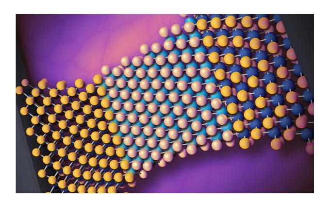
Artist's rendering of a 2D material strategically strained to lie precariously between two different crystal phases. Assistant Professor Stephen Wu from the University of Rochester is using such materials to create hybrid phase-change memristors that offer fast, low-power, and high-density computing memory. Credit: University of Rochester illustration / Michael Osadciw
