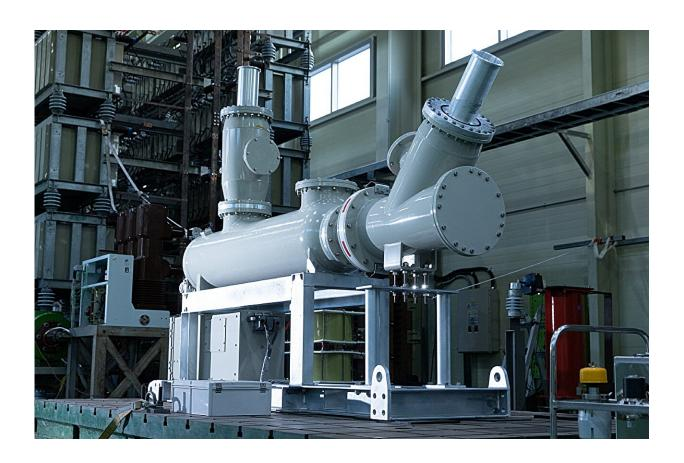
Circuit breaker for high voltage transmission using "K6 eco-friendly insulating gas," which replaces SF6. Credit: Korea Electrotechnology Research Institute
