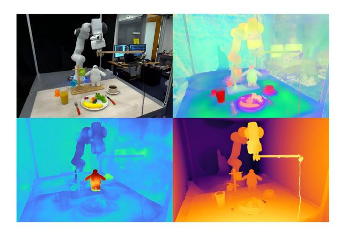
Feature Fields for Robotic Manipulation (F3RM) enables robots to interpret open-ended text prompts using natural language, helping the machines manipulate unfamiliar objects. The system's 3D feature fields could be helpful in environments that contain thousands of objects, such as warehouses. Credit: William Shen et al
