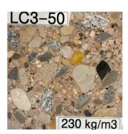
Three LC3-based concretes with varying amounts of cement. As the cement content in the concrete mix decreases, the compressive strength increases. Credit: Franco Zunino
