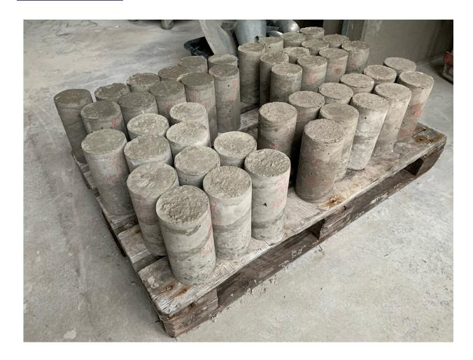
From lab test to prototype: test cylinders of LC3 cement. Credit: Franco Zunino
