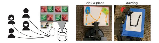
HuGE leverages noisy and asynchronous feedback from multiple non-expert humans to train robot control policies directly on the real world. Credit: *arXiv* (2023). DOI: 10.48550/arxiv.2307.11049
