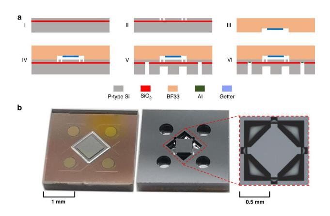
Fabrication of the fabricated PPS with optimal island-diaphragm. Credit: *Microsystems & Nanoengineering* (2023). DOI: 10.1038/s41378-023-00596-y
