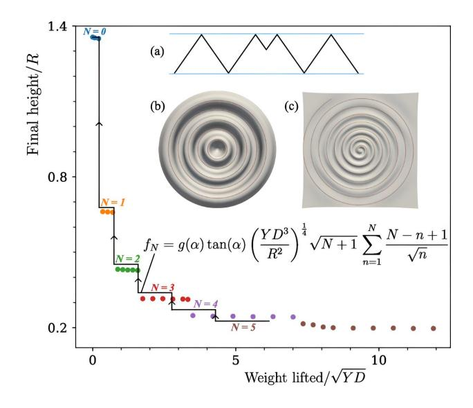
(a) Profile sketch of a concentric-ridged lifter. (b) morphoshell confirms that concentric ridges are roughly equispaced while (c) spiral ridges are
