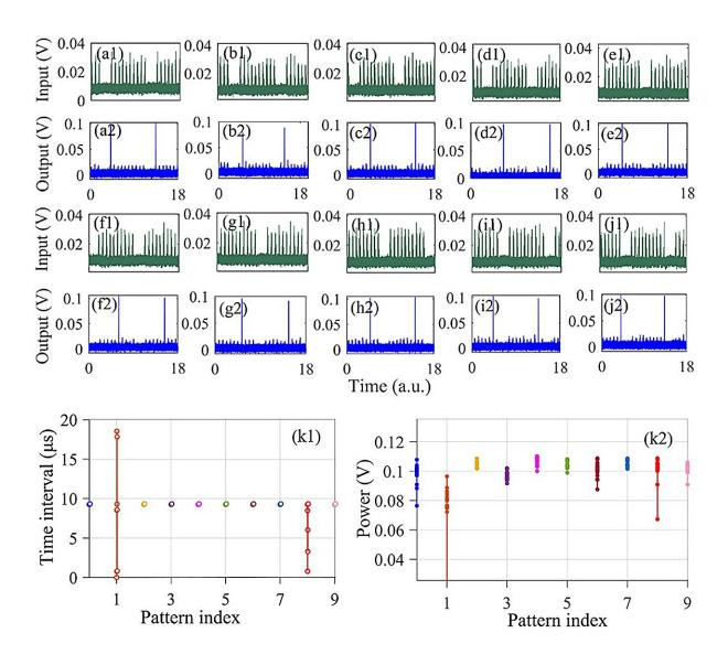
Fig.2. Experimental results of pattern classification based on a DFB-SA laser chip. (a1)-(j1) input spike sequence; (a2)-(j2) corresponding output sequence of
