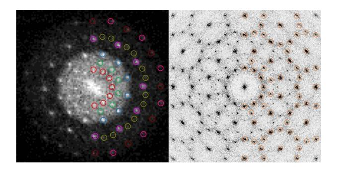
A mathematical tool called a fast Fourier transform maps the structure in a way that reveals the 12-fold symmetry of the quasicrystal. The fast Fourier transform of the electron microscope image of the quasicrystal is shown on the left, while the transform of the simulated crystal is shown on the right. Credit: Mirkin Research Group, Northwestern University, and Glotzer Group, University of Michigan.
