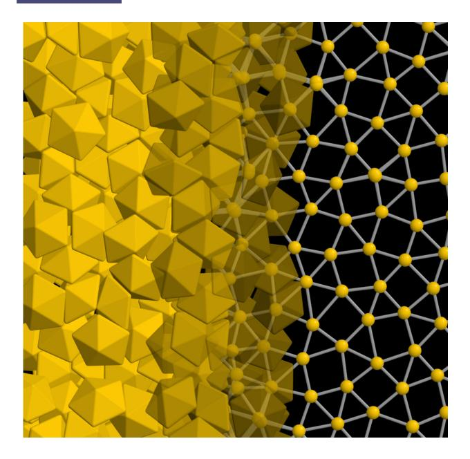
The simulation shows the decahedra packing together into a quasicrystalline structure on the left, with a diagram of the structure on the right. Credit: Glotzer group, University of Michigan.
