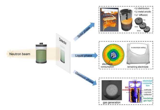
At the upper section of the figure, neutron imaging allows for the observation of lithium dendrite growth and the morphology of electrode. In the middle portion of the figure, neutron imaging enables the monitoring of electrolyte consumption and the infiltration status of the electrolyte. At the lower part of the figure, neutron imaging facilitates the observation of gas generation within coin cell and Li/SOCl<sub>2</sub> battery. Credit: Science China Press
