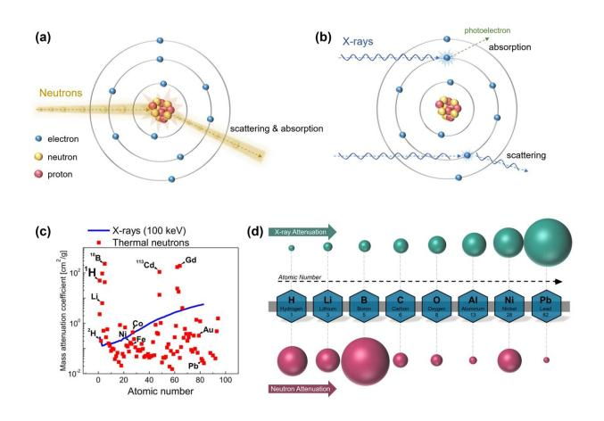
(A) Interaction between neutrons and nuclei. (B) Interaction between X-ray and electrons. (C) Mass attenuation coefficients for thermal neutrons and X-rays (100 keV). (D) Comparison diagram of neutron and X-ray attenuation of different elements. Credit: Science China Press
