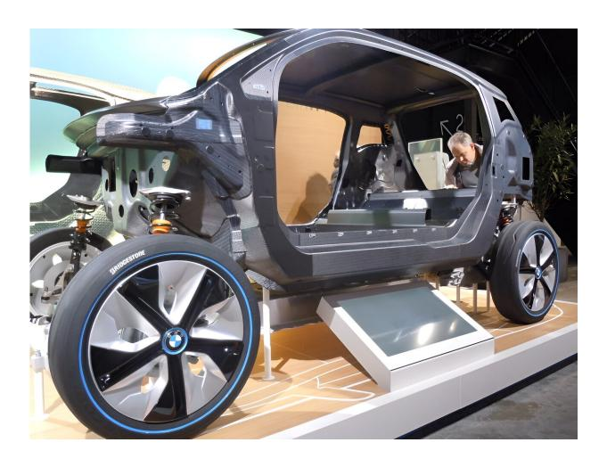
Thanks to their light weight yet remarkable strength, the use of CFRPs in the automobile, aerospace, and renewable energy industries is soaring. However, this means finding effective ways to recycle the waste generated by CFRPs is essential to ensure sustainability in the long term. Credit: LunchboxLarry at Openverse
