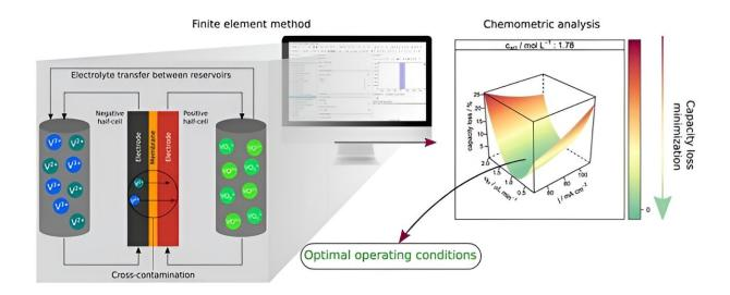
The study involved computer simulations designed to find out how ion leakage between the anolyte and catholyte, called transport loss, leads to battery deactivation. Credit: CDMF The study involved computer simulations designed to find out how ion leakage between the anolyte and catholyte, called transport loss, leads to battery deactivation. Credit: CDMF
