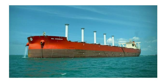
A cargo vessel with Flettner rotors—a modern equivalent to sails. Credit: Norsepower, Author provided
