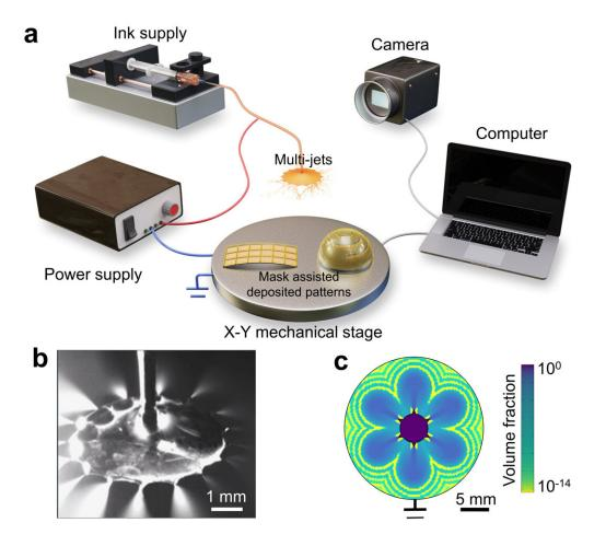
Schematic of electrostatic disc microprinter and multiplexed jetting/tiny droplets from the thin spiny disc. Credit: *Nature Communications* (2023). DOI: 10.1038/s41467-023-42159-9
