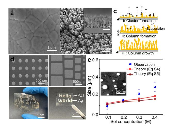
Fabrication of piezoelectric films, micro-patterns and nanoparticles. Credit: adapted from *Nature Communications* (2023). DOI: 10.1038/s41467-023-42159-9
