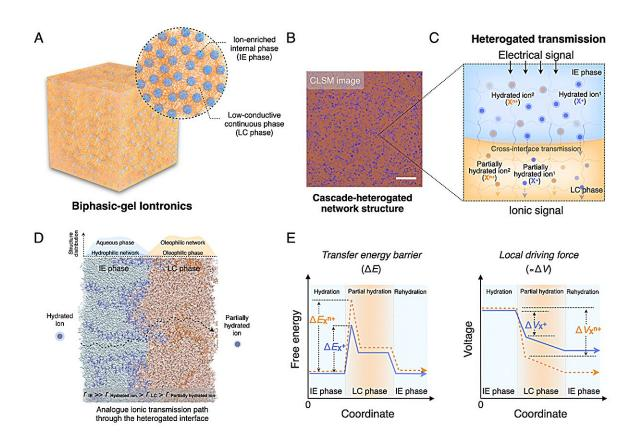
Heterogeneous structures and cross-interface ion transmission of cascadeheterogated biphasic-gel iontronics. Credit: Wen Liping
