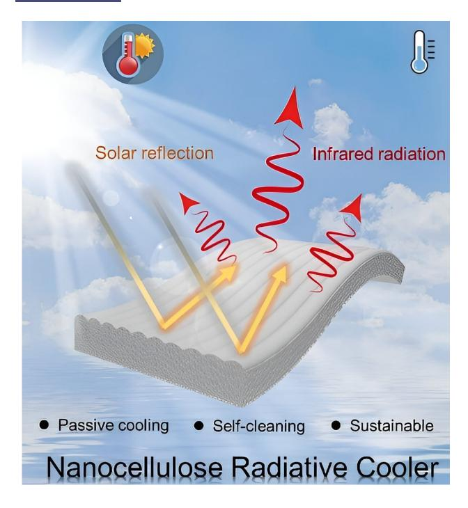
The scheme for passive cooling based on nanocellulose radiative cooler. Credit: Cai, C. et al
