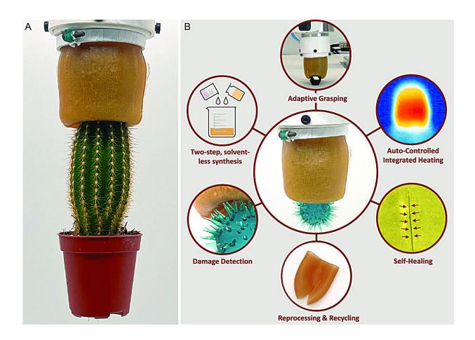
A) SHUG is adaptively grasping a hazardous object (cactus) and B) the highlights of the integrated system. Credit: *Advanced Intelligent Systems* (2023). DOI: 10.1002/aisy.202300223
