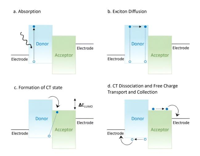
Schematic diagram illustrating the main steps for generation of photocurrent in an OPV. a) photon absorption and formation of an exciton, b) exciton diffusion to the heterojunction, c) Exciton dissociation (via CT state) into free charges at the interface, d) charge transport in the domains and charge collection by the electrodes. Credit: https://kau.diva-
