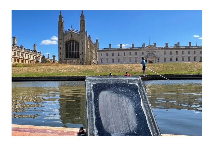
A floating, solar-powered device that can turn contaminated water or seawater into clean hydrogen fuel and purified water, anywhere in the world, has been developed by researchers. Credit: Chanon Pornrungroj/Ariffin Mohamad Annuar
