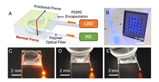
Overview of the OFN sensor. (A) Schematic diagram of the OFN sensing system; (B) Photographs of the output light when the sensor was untouched, (C) subjected to normal force, and (D) subjected to both normal and frictional force. Credit: *Opto-Electronic Advances* (2023). DOI: 10.29026/oea.2023.230076
