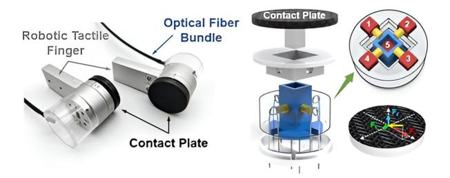
Photograph of two robotic tactile fingers and the exploded diagram of the finger.
