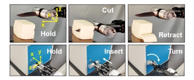
Snapshots during the robot manipulating a knife and a key. Credit: *Opto-Electronic Advances* (2023). DOI: 10.29026/oea.2023.230076
