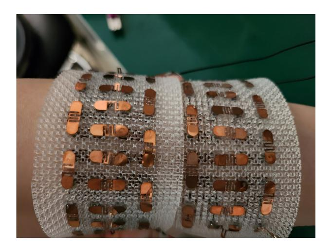
Stretchable/flexible thermoelectric generators using metamaterials. Credit: National Research Council of Science and Technology
