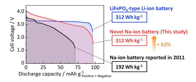
It is possible to incorporate nanopores in hard carbon by using zinc oxide as a template during its synthesis. These pores enable the material to store many more charge carriers, making it a promising electrode candidate for sodium-ion batteries that can reach an energy density comparable to that of LiFePO<sub>4</sub>-type lithium-ion batteries. Credit: Shinichi Komaba, Tokyo University of Science (TUS), Japan
