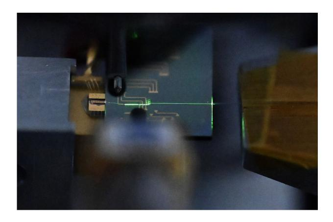
A nanophotonic mode-locked laser built on lithium niobate emits a beam of green laser light. Credit: Caltech
