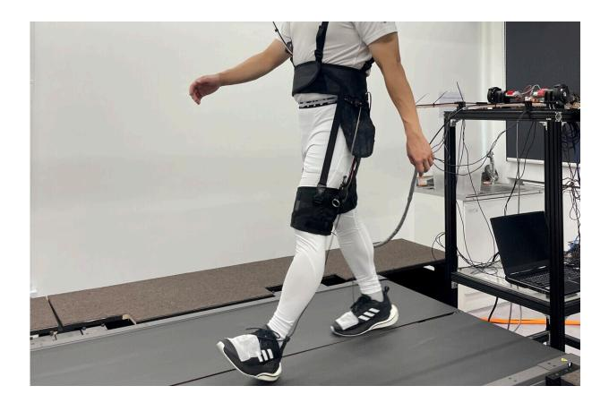
The innovative wearable robot for hip abduction assistance designed at the Assistive and Rehabilitation Robotics Lab at Chung-Ang University. Credit: Park et al.
