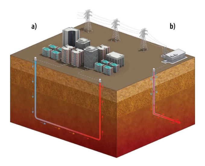
Two common types of closed-loop geothermal systems are (a) u-shaped design (with one or multiple laterals) and (b) coaxial design or "pipe-in-pipe" configuration. Credit: NREL; *Geothermics* (2023). DOI: 10.1016/j.geothermics.2023.102852
