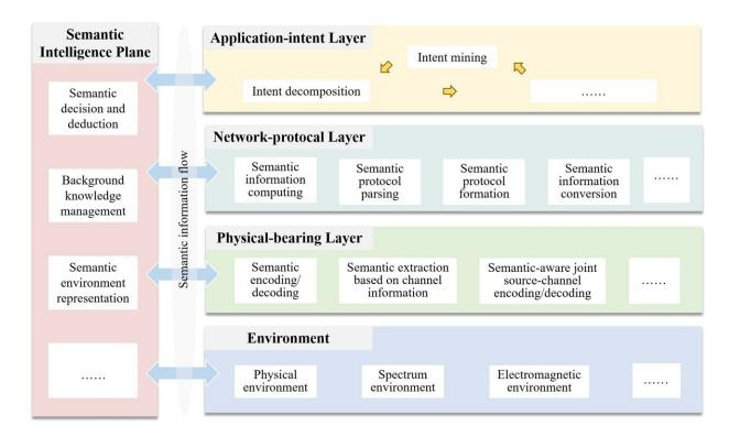
An intelligent and efficient semantic communication (IE-SC) architecture, which composes of an SI plane and three layers: the semantic-empowered physical-bearing layer (S-PB), network protocol layer (S-NP), and application-intent layer (S-AI). Credit: Science China Press
