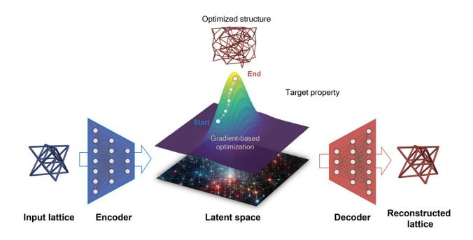
The structure of a metamaterial is encoded in an abstract space. Optimization efficiently improves the design towards the desired properties. A decoder turns the optimized design into a real-world truss structure. Credit: Illustration: ETH Zurich / Li Zheng
