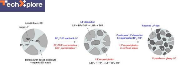
SEI restructuring in borate-pyran electrolyte. Credit: Kwon et al.
