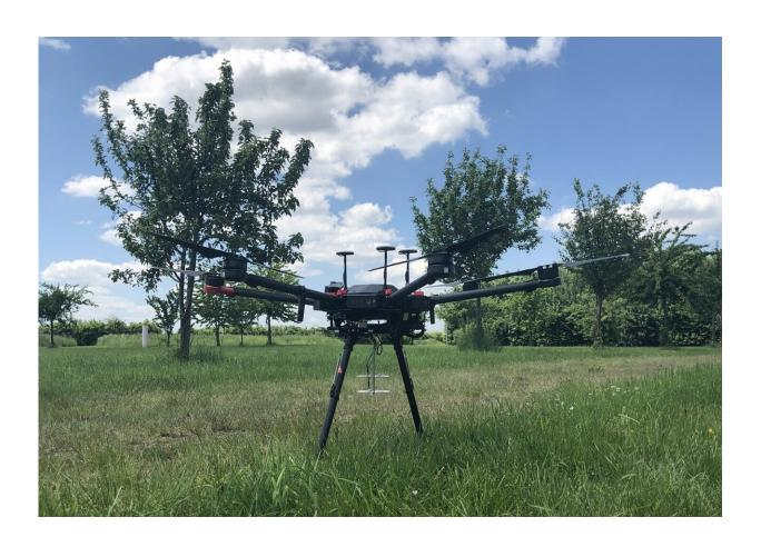
The array of MEMS microphones—known as a crow's nest array—is mounted on a drone. It allows noises such as cries for help and knocking to be detected from the air and their direction to be determined. Credit: Fraunhofer-Gesellschaft
