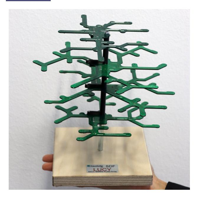
The MEMS microphones are attached in a special geometric configuration in the array and can perceive sound from all directions. The array currently features 48 microphones, but this will increase to 256 in the future. Credit: Fraunhofer-Gesellschaft
