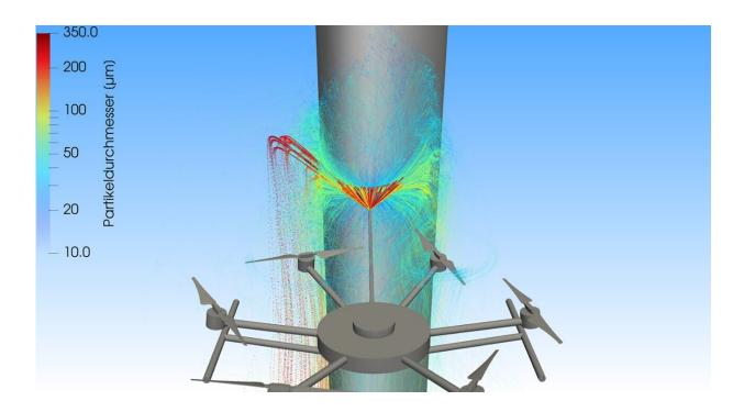
Simulation of coating by means of drone under the influence of wind. Credit: Fraunhofer-Gesellschaft
