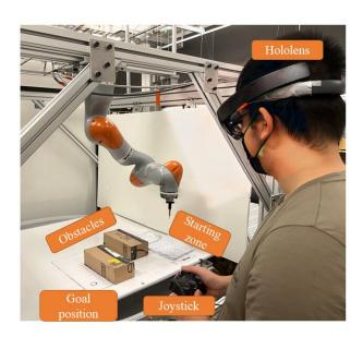
Experimental setup with a user wearing Microsoft Hololens for Visual guidance,
