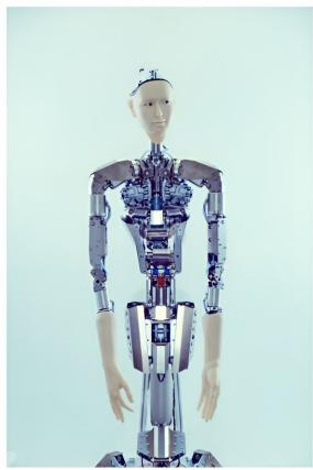
Body of Alter3. The body has 43 axes that are controlled by air actuators. It is equipped with a camera inside each eye. The control system sends commands via a serial port to control the body. The refresh rate is 100–150 ms. Credit: *arXiv* (2023). DOI: 10.48550/arxiv.2312.06571
