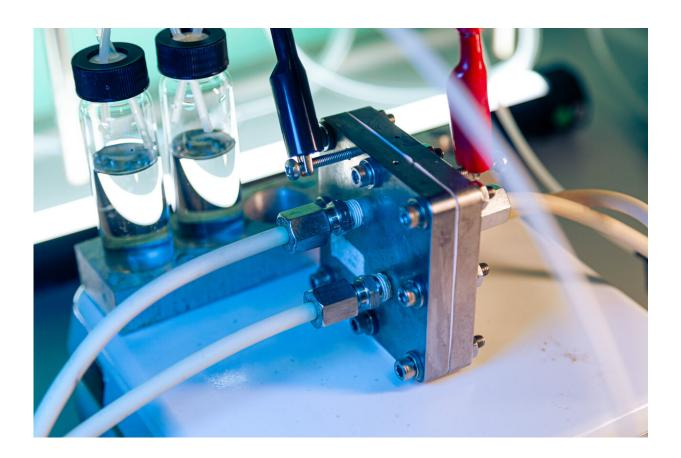
IIT and BeDimensional's researchers used nanoparticles of ruthenium, a noble metal that is similar to platinum in its chemical behavior but far cheaper, to serve as the active phase of the electrolyzer's cathode, leading to increased efficiency of the overall electrolyzer. Credit: IIT-Istituto Italiano di Tecnologia
