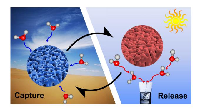
Schematic diagram of the daytime atmospheric water harvesting cycle. Credit: Wang Ruzhu
