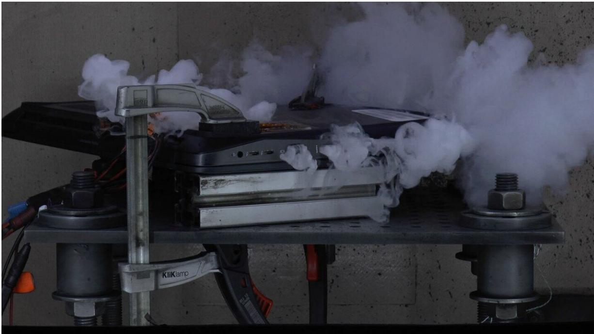
Gas being emitted from a laptop battery during thermal runaway. Credit: Fraunhofer-Gesellschaft
