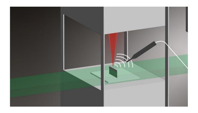
A graphic representation of the experimental setup for listening for printing defects. Credit: 2023 EPFL / Titouan Veuillet—CC-BY-SA 4.0
