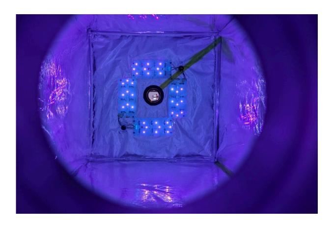
A look inside the MEPS reactor (Methane Eradication Photochemical System), where chlorine atoms are formed by UV light and react with methane gas. Credit: Morten Krogsbøll.
