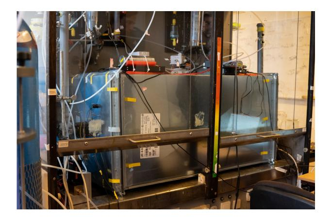
The researchers built a reaction chamber and devised a method that simulates and greatly accelerates methane's natural degradation process. Credit: Michael Skov Jensen, SCIENCE/KU
