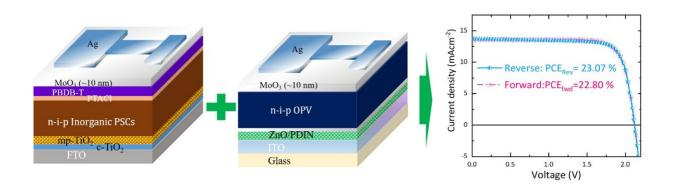
Design of the modified normal "n-i-p" configuration for monolithic 2T-hybrid tandem solar cells devices typically free from complicated processes like atomic layer deposition (ALD) and/or a sputtered interconnecting layer (ICLs) and thermally evaporated C60 ETLs J–V curves of champion hybrid tandem solar cells based on modified configurations in different scan mode. Credit: Dr. Sawanta S. Mali.
